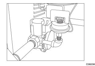
Fig. 29 - LP Low Pressure Switch (Installed)
